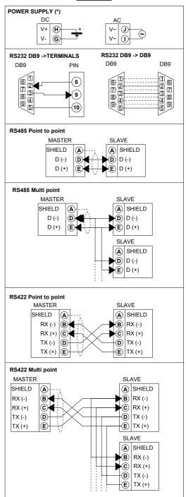
(\*) Note: for UL installation the device must be powered using a power supply unit classified NEC class 2 or SELV
