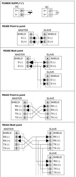
(\*) Note: for UL installation the device must be powered using a power supply unit classified NEC class 2 or SELV
