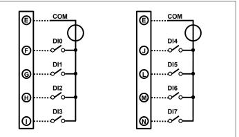
NOTE: the input channels are not isolated between them RELAY OUTPUTS
