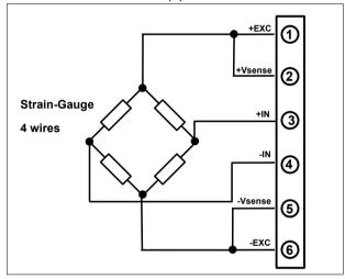
(\*\*) NOTE: in the 4-wires connection, connect a jumper between terminals "1" and "2" and between terminals "5" and "6"
